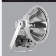
Body, in die-cast Body, in die-cast aluminum painted in gray color. Tempered glass pressed on silicone gasket. Safety insulator block for maintenance operations when opening the cover. Turned reflectors in brightered specular brightened specular aluminum. Fixing bracket in galvanised steel with aiming goniometer in die-cast aluminum painted in
