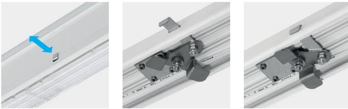
By pushing the mechanism in, the fixture is easily mounted by locking it to the canal. It can be disassembled by pulling the fixture free.
